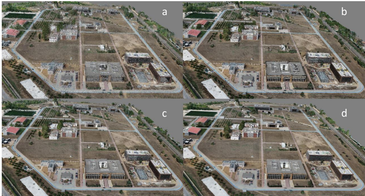
Figure 4. (a) Sparse point cloud, (b) dense point cloud, (c) filtered dense point cloud and (d) 3D textured mesh model of the study area
